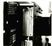
FIG. 8—ONE OF EIGHT high-power precision load resistors mounted on rear of McAdam analyzer.
