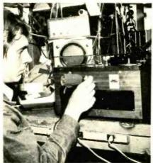
IDENTIFYING A PIECE OF EQUIPMENT with an engraving tool is almost as easy as writing down one's name with a fountain pen. The tool writes on metals, plastics, glass and ceramics. Writing is not easily removed.
