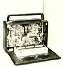
posite function of two dials; the whole number (in MHz) shown on one dial drum and the decimal portion (in kHz) shown on the second. Reception modes include AM, CW and switchable (LSB or USB) single sideband. There are provisions for an external 9-12 volt dc supply, earphone reception and an external antenna (there is a built-in collapsible whip antenna). 11-½ x 7-½ x 3-¾ in.; 9 lbs. 2 oz.; about \$260.00—Giffer Associates, Inc., 52 Park Avenue, P.O. Box 239, Park Ridge NJ 07656.
