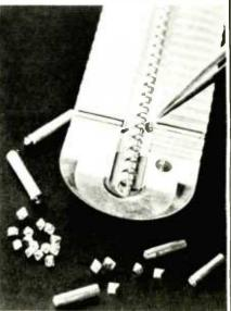
AUTHENTIC DIAMONDS SEPARATE the tiny helix rings from the outer shell of this traveling-wave microwave tube, made at the Waltham, MA, plant of the Raytheon Co. Total weight of the diamonds, used because they are excellent heat conductors as well as electrical insulators, is about four carats per tube.
