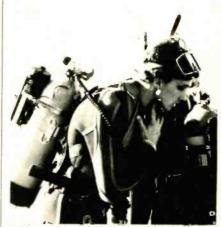
UNDERWATER COMMUNICATION IS EASY with the units shown strapped to the air tanks. Voice communication is feasible up to 165 feet.
