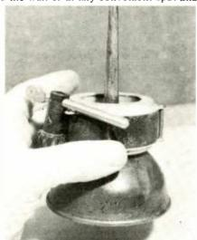
hold an assortment of metal items. It is especially useful to hold squirt cans — usually made of copper-plated sheet iron since the spout of the can may be inserted through the center of the ring from the bottom where it will be held securely until needed. For greater security spring-mount the magnet in some way to resist shock and vibration. — Glen F. Stillwell
